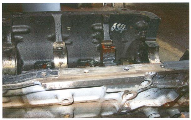
Below is another example depicting main journal damage, crankshaft damage and engine serial number in a single photo.
